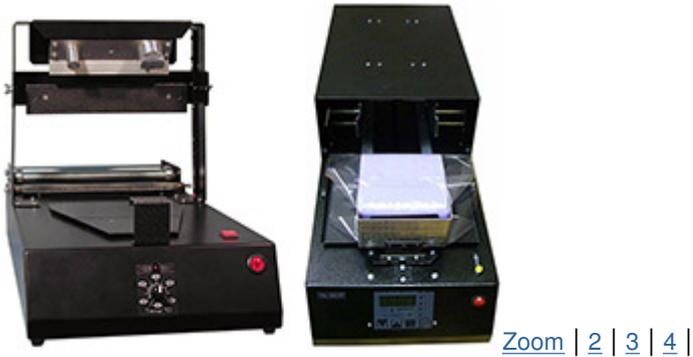
Machine is intended for semi-automatic packing of different items in a polypropylene film. In factory it is tuned up for semi-automatic packing of napkins. If you want to pack other items on this machine in semi-automatic mode then you will have to install other [replaceable module](#) for required item and install film of [other width](#).
